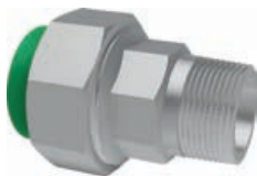
G 8547gB PP-RCT-V2A Ü-Verschraubung AG-keg Flachdichtring-EPDM 20°C/1.0MPa grün PP-RCT-Stainless steel Transition-Union male-thread-con flat-gasket-EPDM 20°C/1.0MPa green
